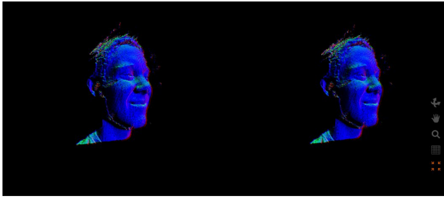
Figure 4.6 Visualization of a 3D frame after split-screen stereo has been applied; there is one view for each of the user’s eyes. When visualized inside of an Oculus Rift, two images appear to be one 3D image.
