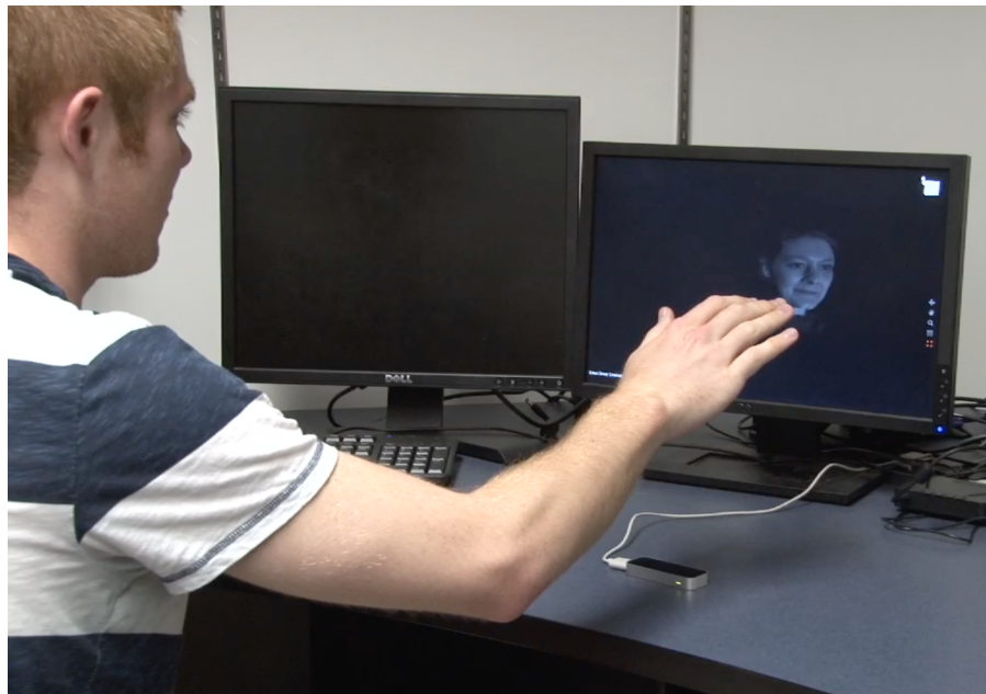
Figure 4.12 The author interacts with 3D video in the visualization system using the Leap Motion Controller. His hand movements control the virtual camera's view of the 3D geometry. Original photograph taken by Karpinsky (2013b).
